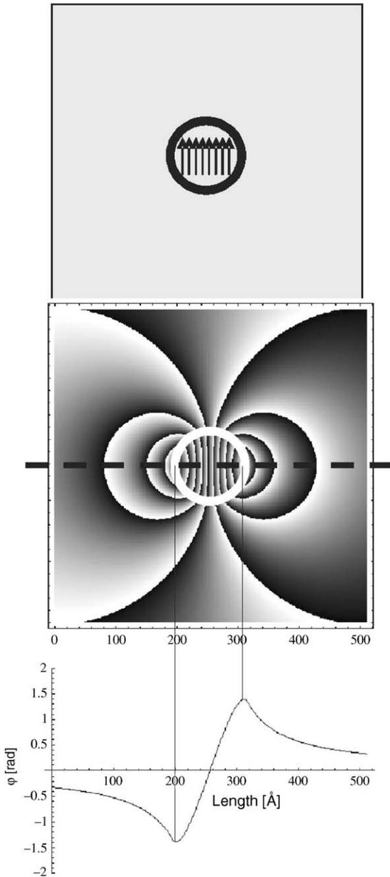
Fig. 7. Simulated phase distribution around a homogeneously magnetized sphere as reconstructed from a hologram. Top: sphere of 30 nm radius with indicated inner magnetic-field of 1 T. Middle: phase distribution with contours. Bottom: linescan of phase along broken line.
