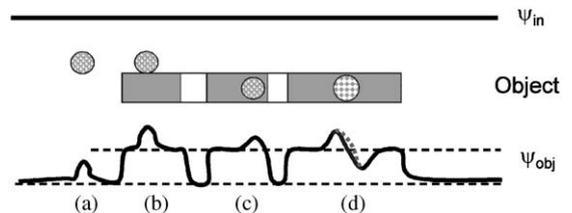
Fig. 4. Scheme how the electron phase of the beam can be affected by different electric and magnetic objects which are either free standing or embedded within a crystal. Electron phase modulation by an electric sphere (a), electric sphere on top of a foil (b), and embedded in a foil (c), separated by holes. (d) shows a sphere homogeneously magnetized perpendicularly to drawing plane without (solid line) and with electric potential (broken line).
