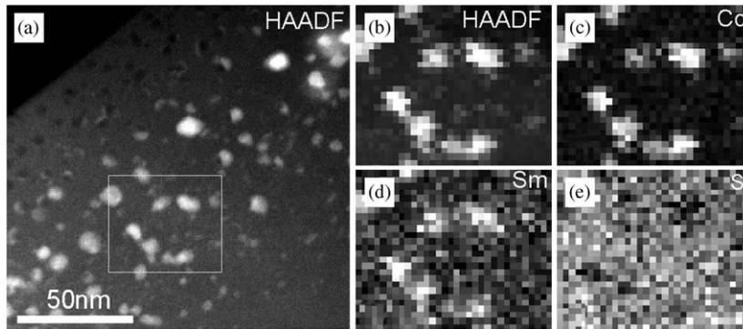
Fig. 12. HAADF-STEM images (a, b) and EDX-STEM maps of nanocrystals created after Co and Sm-ion implantation in 4H-SiC and annealing. (a) overview HAADF-image showing the region (marked) for the EDX-STEM analysis. (b) HAADF-STEM image, (c) Co, (d) Sm and (e) Si-EDX maps (the selected area was scanned with 1.3 nm wide raster). The nanocrystals always show an increase of the Co and the Sm-signal, while the Si-signal in the nanocrystals is clearly lower than in the matrix.
