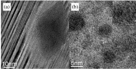
Fig. 3.  $\text{Co}_2\text{Si}$ -nanocrystals in 4H-SiC surrounded by onion-like carbon in cross-sectional view projected along  $[11\bar{2}0]$  4H-SiC (a) and in plane-view projected along  $[000\ 1]$  4H-SiC; the insert magnifies the inner part of the onion, showing the nanocrystal (b). The distance between the single shells is 0.34 nm, which corresponds well to the interplanar distance of graphite.
