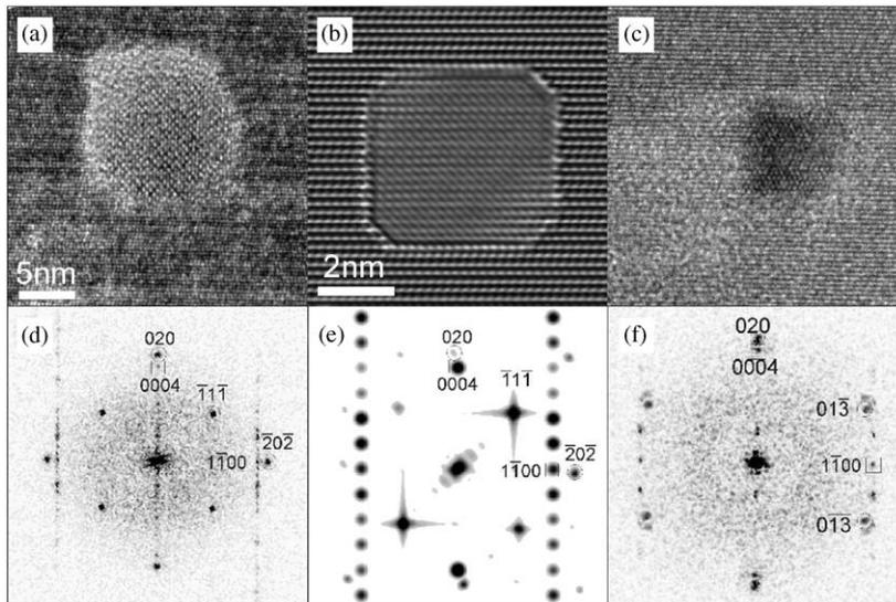
Fig. 2. HRTEM images of  $\text{Co}_2\text{Si}$ -nanocrystals in 4H-SiC created after Co-ion implantation and annealing viewed along  $[11-20]$  4H-SiC; experimental images (a, c) and the corresponding diffractograms (d, f); calculated image (b) and calculated diffraction pattern (e, the asymmetries of intensities are caused by inaccuracies during the tilting and embedding processes (see 2. Experimental)). Reflections of nanocrystals are encircled, reflections of 4H-SiC are boxed.
