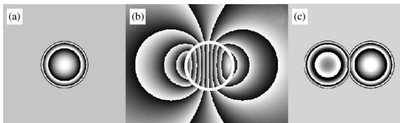
Fig. 6. Simulated phase distributions inside and outside spherical particles with (a) electric potential and (b) inner magnetic field, (c) shows an electric dipole, e.g. given by a sphere close to a hole; this could mimic a magnetized sphere hence lead to misinterpretation. However, in contrast to (c), (b) reveals the typical stray-field reaching far out from the particle, which is characteristic for a magnetized sphere.
