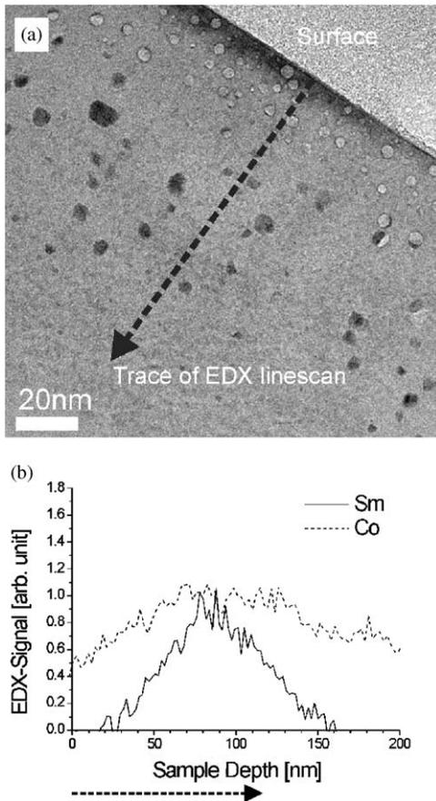
Fig. 10. (a) Bright field image of Sm/Co-ion implanted 4H-SiC. The area selected for EDX-linescan analysis is visualized by the arrow. (b) Element distribution of Co and Sm with maxima at a depth of around 100 nm showing a much broader profile for the case of Co.
