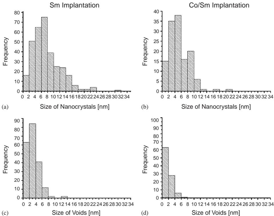
Fig. 14. Size distribution of nanocrystals and matrix voids for the Sm and Co/Sm implantation. It can be easily seen that nanocrystal size are comparable for this two implantations.
