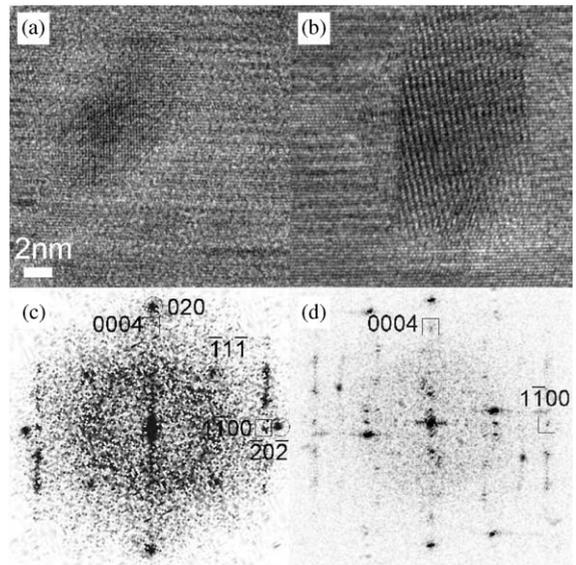
Fig. 11. [11–20] HRTEM images of nanocrystals formed in 4H-SiC after Co/Sm-ion implantation and corresponding diffractograms. (a, c)  $\text{CoSi}_2$ -nanocrystal formed in the surface-near region. (b, d) Nanocrystal of more complex structure formed in the surface-far region. Indexed reflections of nanocrystals are encircled, reflections of 4H-SiC are boxed.
