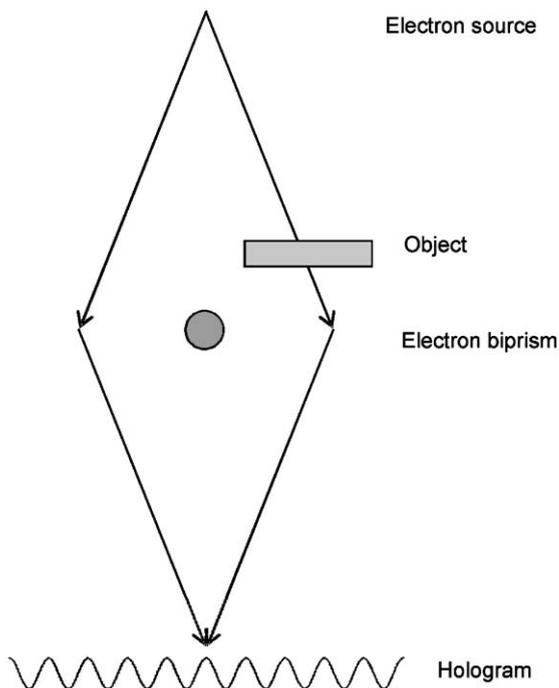
Fig. 5. Scheme for producing an electron hologram. The object wave modulated by the object structure (right) interferes with the plane reference wave (left) to form a hologram.
