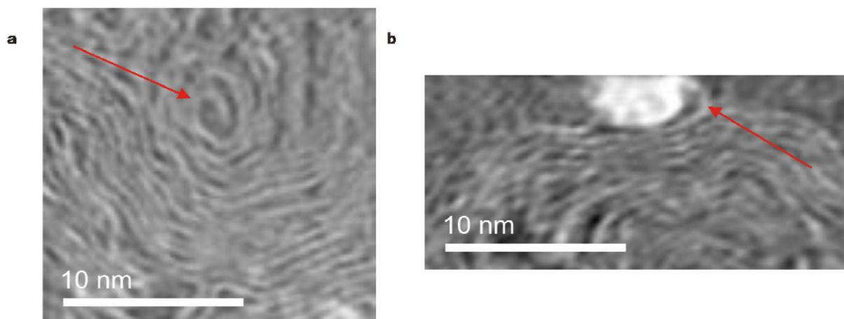
**Figure 2.** Cross-sections of the reconstructed tomogram revealing interesting features of the carbon soot particle: (a) shows a spiral-shaped graphitic plane in the interior of the soot particle; (b) shows a carbon monolayer covering a Pt-particle positioned on the outer surface of the soot particle.
