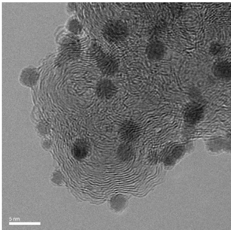
**Figure 1.** One of 46 tilt-images in total ranging from  $-66^\circ$  to  $+69^\circ$  ( $3^\circ$  tilt increment) showing variously formed graphitic planes composing the interior structure of the soot particle acting as a support for the catalytically active Pt particles.
