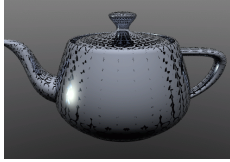
Figure 4: False surface intersection reported by Newton iteration, when the starting point is not sufficiently close to the fix point.
