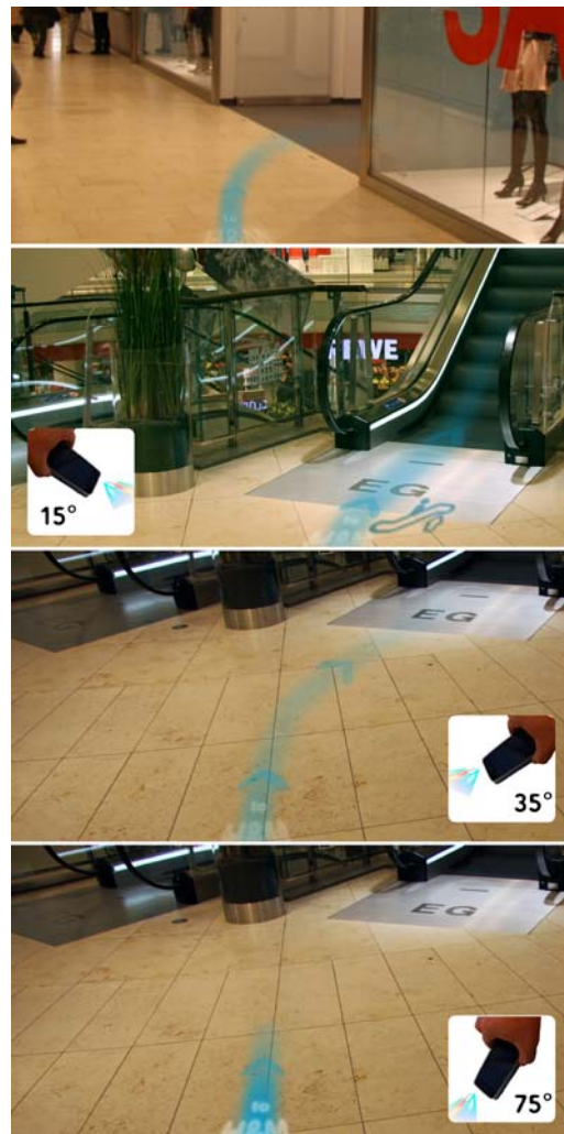
Figure 3: Envisioned navigation. From bottom to top: (1) The user follows the blue line. (2) She explores the line further to see which escalator to take. (3) The line “runs up” the escalators and (4) leads directly into the desired shop.
