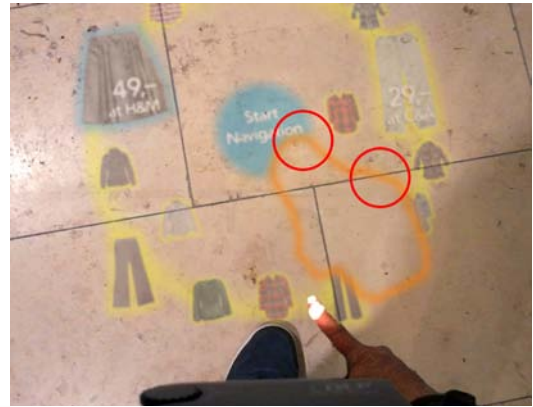
Figure 2: The user interacts with his radar of recommendations through the shadow of his finger. The orange outline shows the shadow, the left red circle the fingertip that, for clicking, can be changed independently of the finger's middle knuckle (right circle) or the rest of the hand's shape.
