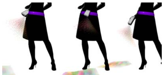
Figure 1: The projector is worn at different locations on the belt (left and middle) and can optionally be taken into hand to change the angle of the projection (right).
