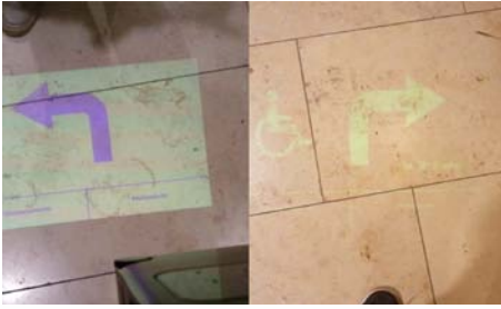
Figure 5: Lighting conditions in a nearby shopping center. Left: Blue arrow with yellow background in dark environment (ca. 200 lux). Right: Yellow projection in comparable bright environment (ca. 400 lux). Projector: Aiptek Pocket Cinema
