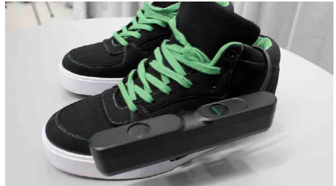
Figure 4. ShoeSense [4]: A shoe with an attached depth camera.
