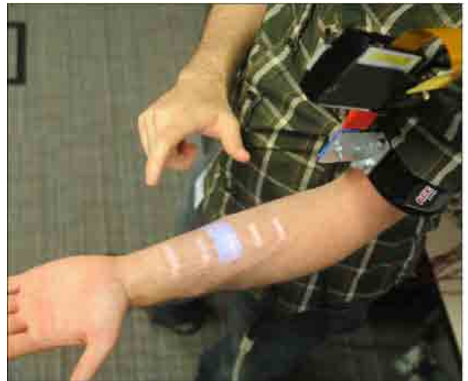
Figure 6. Skinput [11]: The sensing armband augmented with a pico-projector which allows to see the interactive menu on skin.
