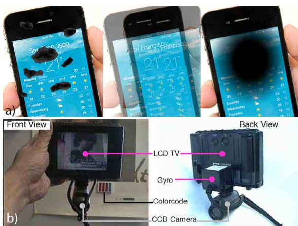
Figure 2. (a) By overlaying and distorting the user’s view an experience of visual impairment like Glaucoma can be generated [5]. (b) Real-world images are captured by a camera on the back and presented to user on the front-screen to create a magnifying-glass metaphor [33].
