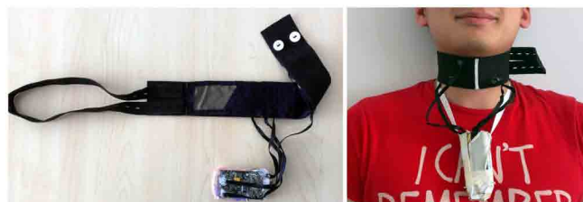
Figure 10. The prototype of the capacitive neckband [13].
