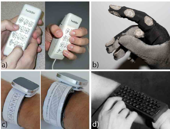
Figure 4. (a) The Twiddler uses chording for text input [30]. (b) Argot , a wearable one-handed keyboard glove [31]. (c) A touch-sensitive wristband for text entry [13]. (d) A forearm keyboard used in a study by Thomas et al. [22].
