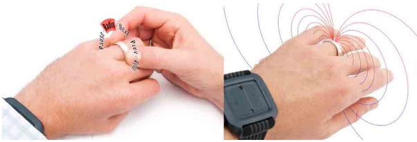
Figure 1. Nanya [1]: A technique using the magnetism of a ring to produce input for a wearable device. For this the receiver on the arm can interpret the changes in the magnetic field.
