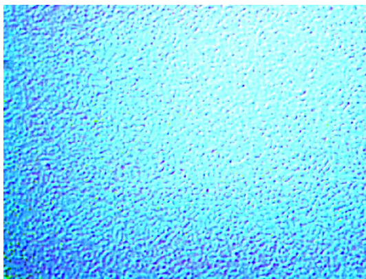
Fig. 4: Nomarsky contrast micrograph of the sample X19 at 1000 magnification. Due to the relaxation the surface is rough.
