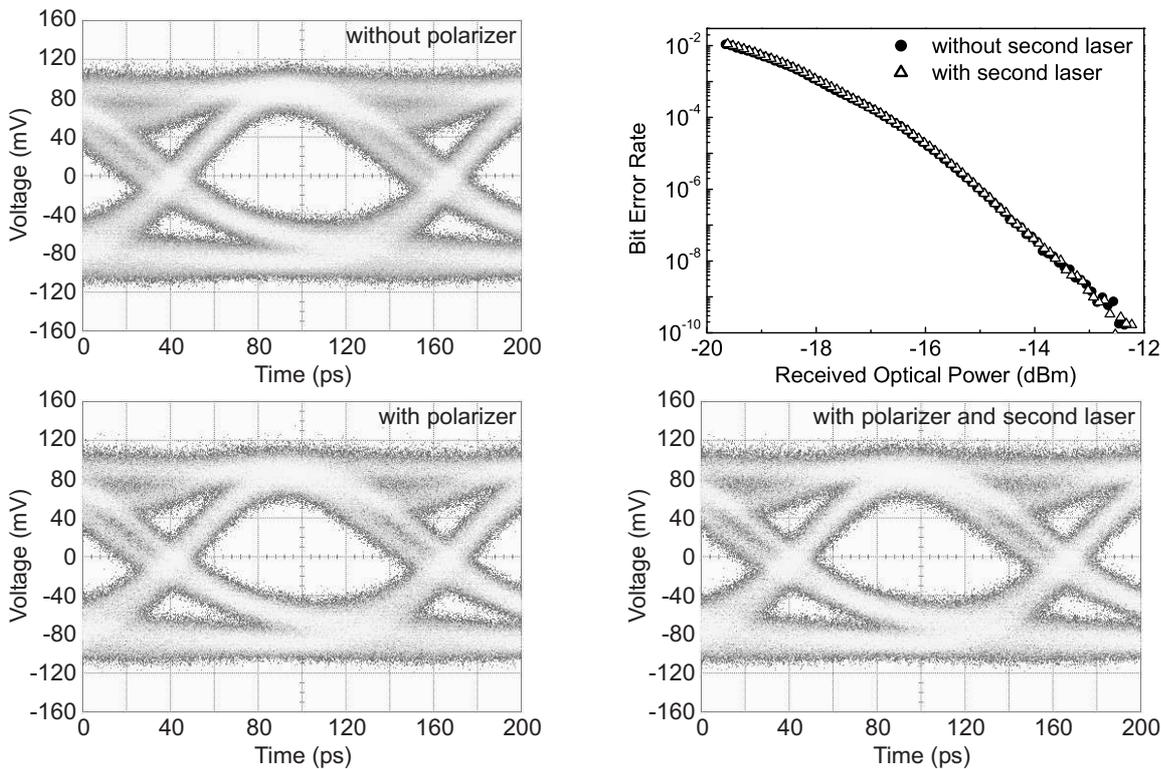
**Fig. 3:** Optical eye diagrams of surface grating VCSELs at a data rate of 8 Gbit/s. Channel 1 VCSEL before (top left) and after (bottom left) the insertion of the polarizer in Fig. 2 as well as with the orthogonally polarized channel 2 VCSEL switched on (bottom right). Bit error rate characteristics corresponding to the bottom left and right eye diagrams (top right).
