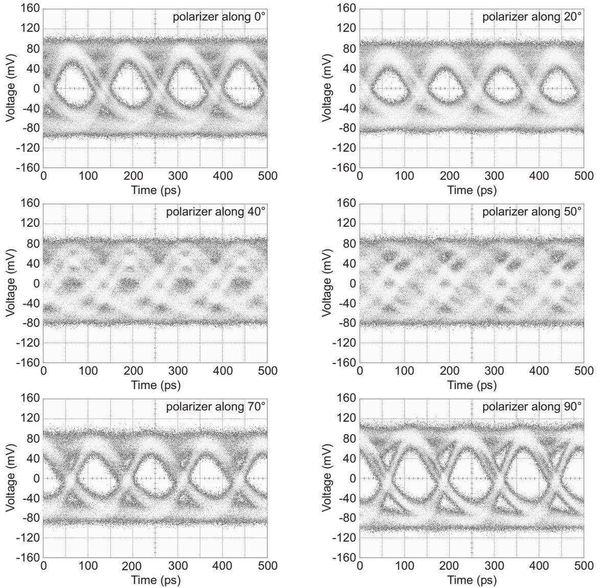
**Fig. 4:** Optical eye diagrams recorded for a free-space polarization division multiplexed optical link using two orthogonally polarized grating VCSELs that are simultaneously modulated at 8 Gbit/s data rate. The orientation of the polarizer is indicated in each graph. The VCSELs and the modulation conditions are the same as in Fig. 3.
