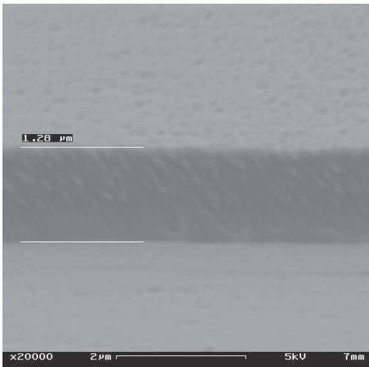
**Fig. 3:** SEM picture of mesa side flank (HVPE sample), height  $\approx (1.2 \pm 0.1)\ \mu\text{m}$ .
