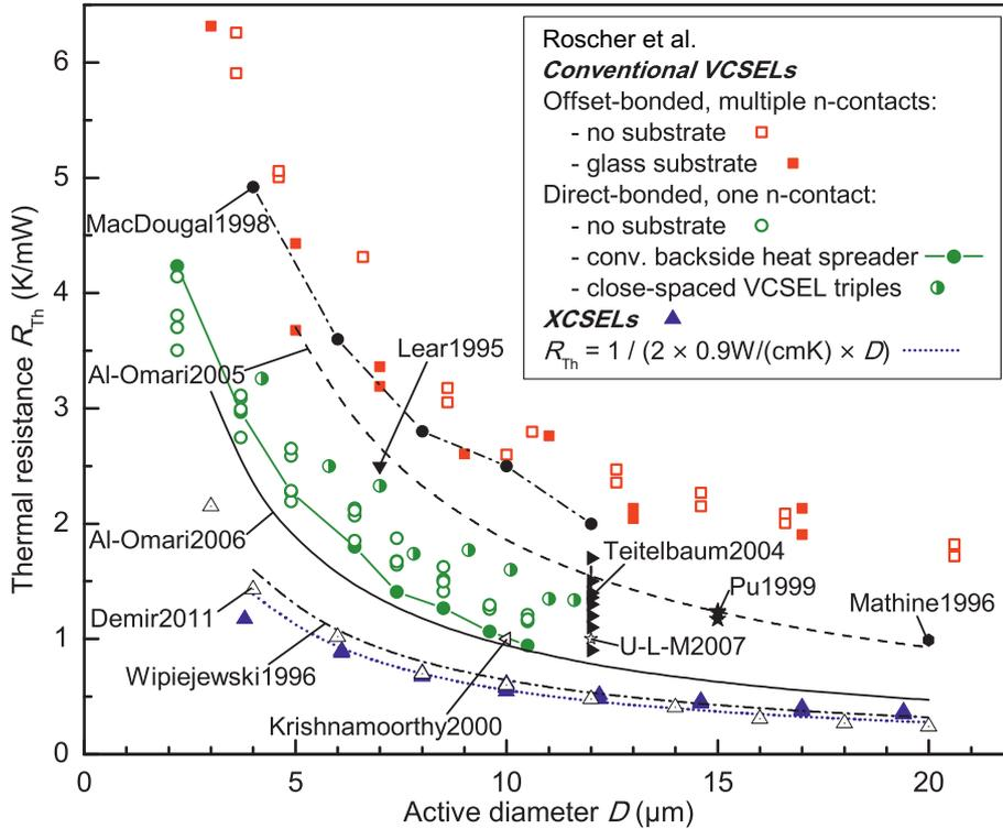
**Fig. 5:** Overview of thermal resistances achieved for many device configurations. For comparison, data from previous works is included, indicating the first author and year of publication for convenient reference. Corresponding publications are provided in the text.
