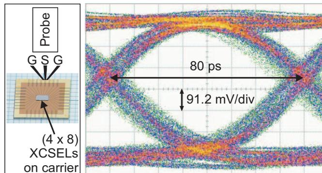
**Fig. 7:** Photograph of the XCSEL array on a carrier fanout chip with a schematic contact arrangement of a microwave probe (left) and 12.5 Gbit/s eye diagram for modulation with a  $2^7 - 1$  word length pseudorandom bit sequence (right).
