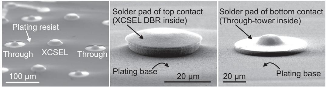
**Fig. 4:** SEM images of about  $5\ \mu\text{m}$  thick plated solder pads wrapped around the top parts of the VCSELs and through-connections. In the left-hand image the pads are still embedded in the plating resist while in the two images to the right the resist has been removed.
