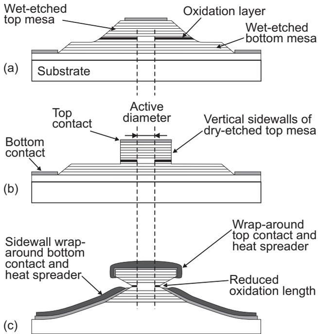
**Fig. 1:** (a) Conventional wet-etched VCSELs. (b) Conventional dry-etched VCSELs with vertical top mesa sidewalls. (c) XCEL exhibiting the characteristic X-shaped outline.
