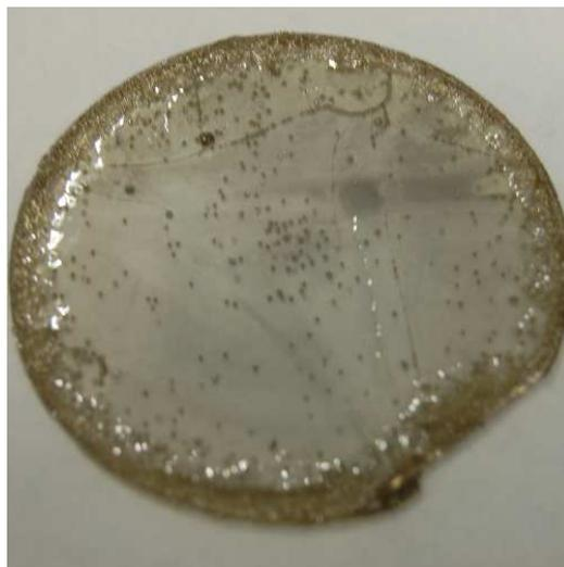
**Fig. 4:** Photography of whole self-separated, freestanding GaN-wafer.
