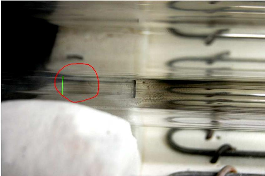
**Fig. 4:** Photograph of the 8 mm glass tube with iron deposits (inside the circle). The bright line marks the position of the shortening. The larger transport tube also shows some depositions.
