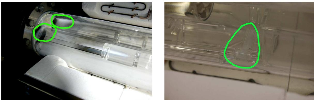
**Fig. 3:** Photographs of the reactor inlets (left) and the quartz tube/gas-mixing chamber junction (right) during an ammonium-chloride haze experiment to determine the maximum possible flow inside the ferrocene doping channel. Bright lines are enclosing ammonium-chloride depositions.
