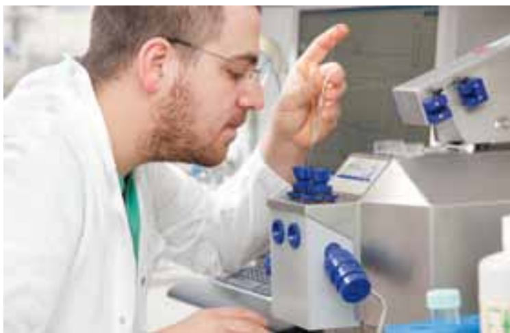
Addition of substrate during high resolution respirometry determination of the activity and the coupling status of the mitochondrial respiratory chain.
