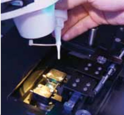
Computer-controlled cell stretch device mounted on the stage of an inverted microscope. Lung cells are grown on the silastic membrane on top of the objective.
