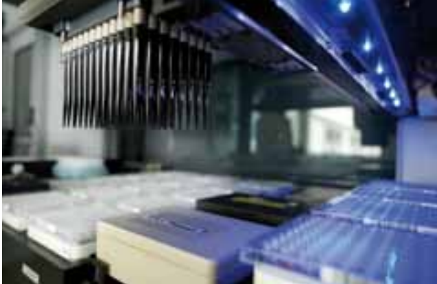
Robotic work station for high throughput HLA typing using a CE-marked kit developed by the Institute of Transfusion Medicine Ulm for sequence-based HLA-typing.
