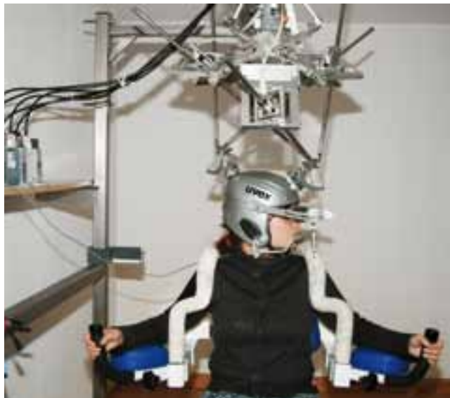
Force-Feedback-System for sensor-motoric neck muscle training after spine injury.
