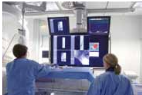
Intracranial interventional procedure performed with a large 60" LCD viewing display. Both interventional accuracy and radiation dose exposure are reduced due to the large area display unit.
