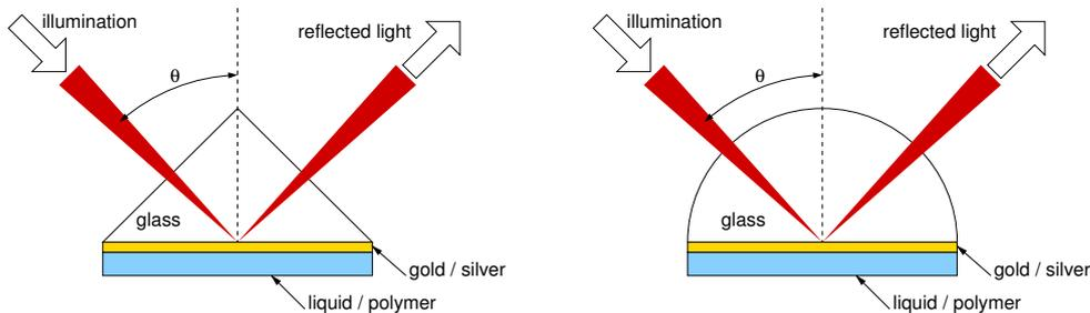
Figure 1: (left) SPR setup using a  $90^\circ$  prism. (right) SPR setup using a cylindrical prism.
