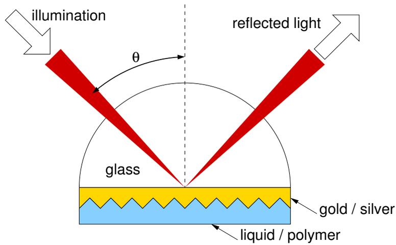
Figure 2: SPR setup for a grating
