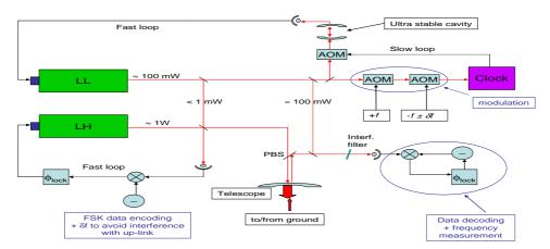
Fig. 3-1: Principle of the laser set-up for DOLL
