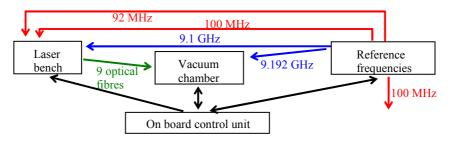
Fig. 3.1.-1: Atomic accelerometer subsystems
