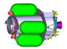
**Fig. 4-2:** Potential propulsion module for SAGAS based on the EUROSTAR/LISA Pathfinder Propulsion Module heritage
