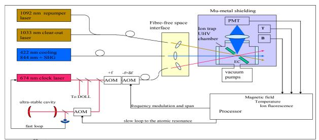
**Fig 3.3.-1:** <sup>88</sup>Sr<sup>+</sup> ion clock system architecture: EO, electro-optic modulator; AO, acousto-optic frequency shifter; det, detector; PMT, photo-multiplier; SHG, second harmonic generation; EC, end-cap trap; T, temperature sensor; B, magnetic field sensor. Redundant laser units not shown, nor control lines for active unit monitoring and redundant unit activation after major fault diagnosis, nor standard monitoring and control lines.
