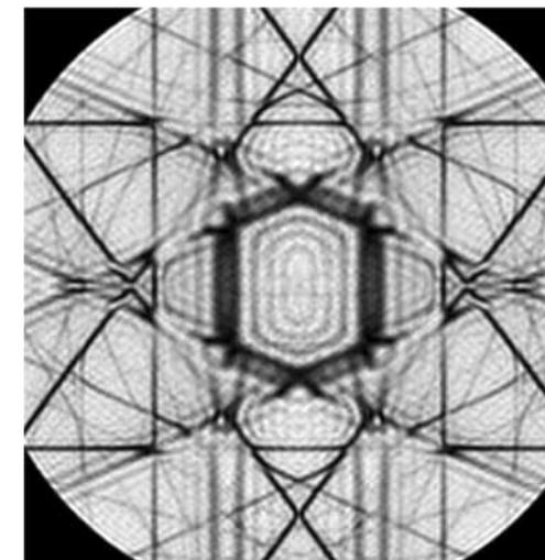
Image 2: Wide angle convergent beam electron diffraction on InGaAs in the [012] projection. Not only are the pictures aesthetically pleasing, the fine lines also enable scientists to determine lattice constants locally and with the greatest precision.
