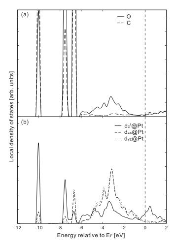
FIG. 4: Local density of states calculated by projection of wave functions onto the atomic orbitals in the case of the CO adsorption at the top site of the 2-ML thick surface alloy III, i.e. the Pt/Pt<sub>0.33</sub>Au<sub>0.67</sub>/Au(111) surface, (a) for the C and O atoms and (b) for the three *d* orbitals  $(d_{z^2}, d_{zx}, \text{ and } d_{yz})$  of the Pt atom the CO molecule is bound to.
