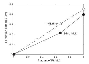
FIG. 2: Surface alloy formation enthalpy  $\Delta H$  calculated as the difference in the total energy between a Pt/Au(111) electrode and a Au(111) electrode with corresponding number of Pt and Au atoms exchanged from a bulk reservoir (see eq. (2)).
