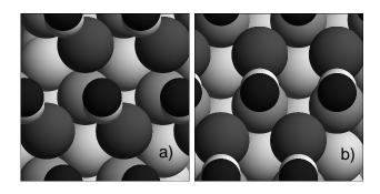
FIG. 2: Adsorption geometries for CO on Pd(210). O is drawn in black, C in white, the Pd atoms are shaded in gray. The left panel (a) illustrates the final adsorption geometry of CO at site E, the right panel (b) at site C. In both cases, the bridge-bonded, inclined CO geometry is clearly visible.
