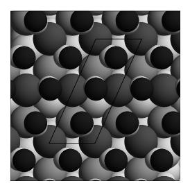
FIG. 3: Adsorption geometry of CO/Pd(210) at a coverage of  $\theta = 1.5$ . The color coding is identical to the one used in Fig. 2. The CO molecules are (approximately) located at sites E, B, and C' (from bottom to top). The  $(1 \times 2)$  surface unit cell is also shown.
