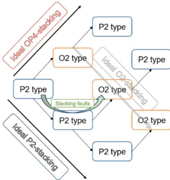
Figure 9: Schematic figure of the formation of P2, O2 and OP4 structure.
