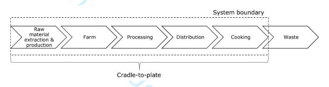
Figure 2 Streamlined illustration of a generic cradle-to-plate Life Cycle Assessment as used in the presented service-learning LCA course. Modeling the ecological impacts of the generated waste and/or recycling processes is outside the scope of the study.
