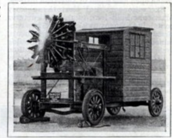
This movable testing stand for airplane engines, developed at Roosevelt Flying Field, will travel seventy miles an hour.
