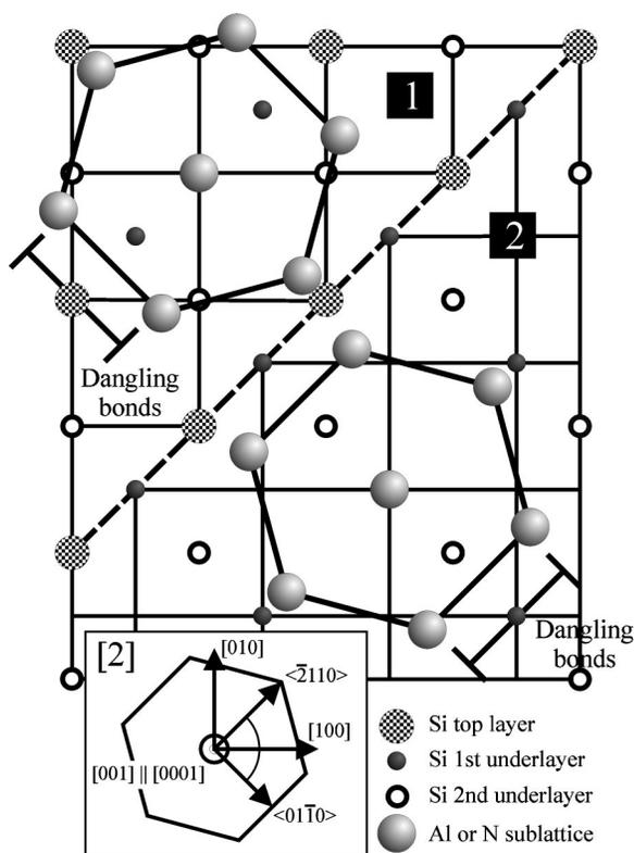
FIG. 4. Atomic arrangement for the heteroepitaxial nucleation of 2H-AlN on the Si(001) surface. The AlN nuclei with different orientations are formed on neighboring terraces (1) and (2) separated by SASB according to the Si dangling bond-directions.
