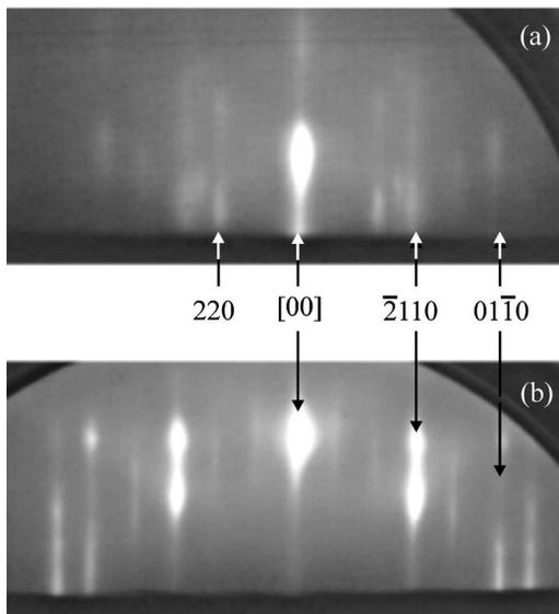
FIG. 1. RHEED observations: (a) a superimposed pattern from the Si(001) surface under AIN nucleation with a superposition of 220 Si, 01 $\bar{1}$ 0 AIN<sup>1</sup>, and  $\bar{2}$ 110 AIN<sup>2</sup> reflections; (b) 3 $\times$ -reconstructed pattern from a 200-nm-thick AIN film surface demonstrating a superposition of the reflections from both domain types.
