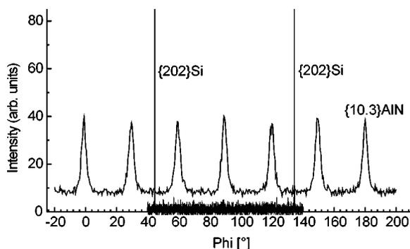
FIG. 2. XRD  $\Phi$  scan demonstrates a 12-fold crystallographic symmetry of a 500-nm-thick AIN film grown on Si(001). The  $a_1$  axis of AIN and  $a_1$  axis of Si have a  $15^\circ$  angular shift.
