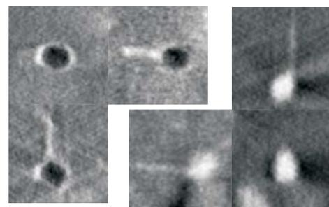
Stripes attached to nanovoid and nanocrystal - X-sections of tomographic reconstruction.
