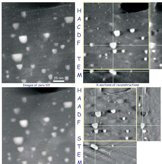
As can be seen: Reconstructed nanocrystals obtained by Z-Contrast TEM and -STEM Electron Tomography give about the same result. The methods do not differ significantly in resolution.
