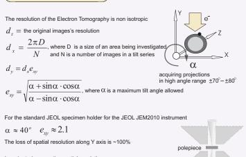
In order to improve the spatial resolution, special specimen holder and grids were developed, that allows
