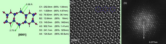
(a) The image was taken at 620 k magnification, corresponding to a sampling rate of 0.029 nm/ pixel. Close examination reveals a different orientation relative to the above one. (b) Fourier components of the structural image extend into the sub-ångstrom region as indicated by arrow.
