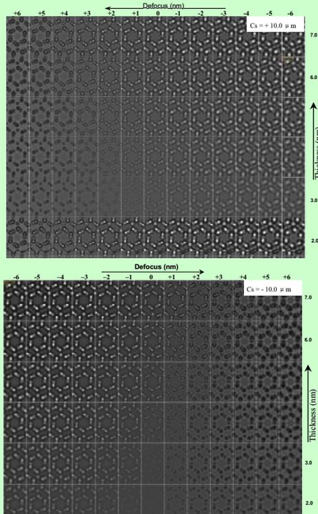
The calculated images show that under  $C_s$  and a small overfocus (indicated by  $\circ$ ), Si-N dumbbells and individual nitrogen columns are well resolved over a large range, and presenting 'bright' white atoms on dark background. Asymmetrical image contrast demonstrates the non-linear contributions.
