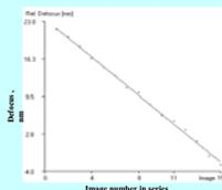
Defoci measured for individual micrographs from the through-focus series of image in (a). Value of average focal step size (linear fit): -1.72  $\pm$  0.02 nm.
