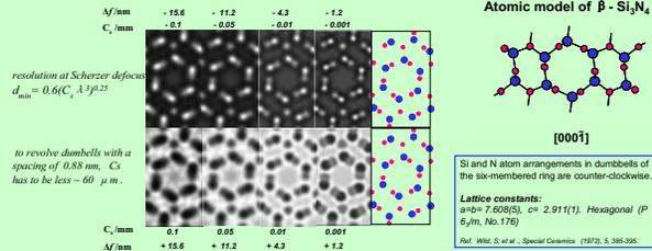
I-B. Image calculation under the symmetrical  $C_s$  and defocus
