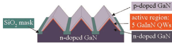
Figure 1 (online color at: www.pss-a.com) Schematic view on LED structures grown on the side facets of n-doped GaN stripes grown by selective area epitaxy using SiO 2 as mask material.
