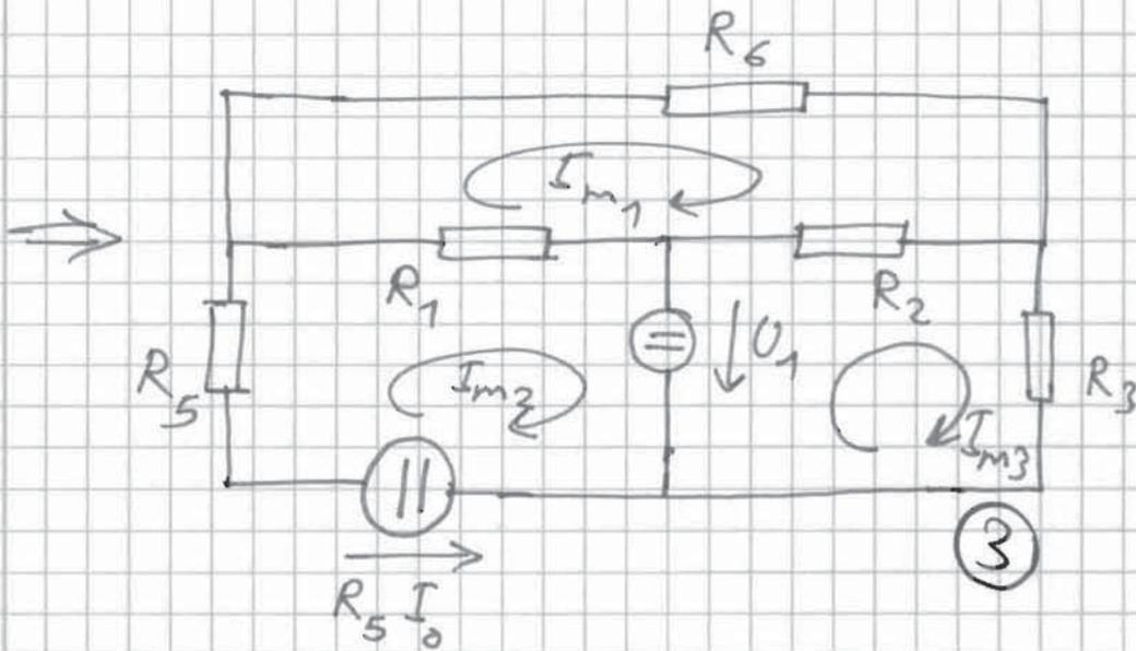
$$\text{MR1: } R_6 I_{m1} + R_2 (I_{m1} - I_{m3}) + R_1 (I_{m1} - I_{m2}) = 0 \quad (1)$$
