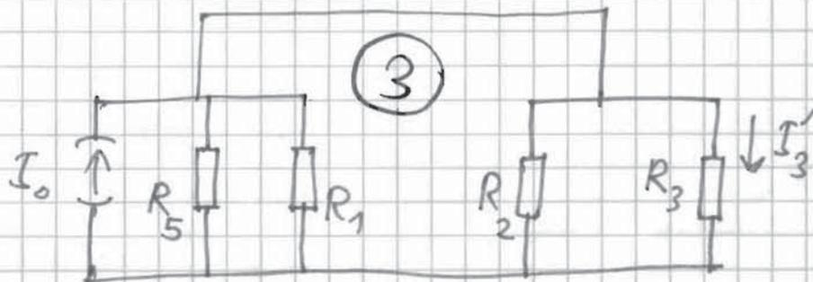
$$I'_3 = \frac{(R_5 \parallel R_1 \parallel R_2)}{R_3 + (R_5 \parallel R_1 \parallel R_2)} I_0 = \frac{(2R \parallel \frac{R}{2})}{R + (2R \parallel \frac{R}{2})} I_0 =$$
