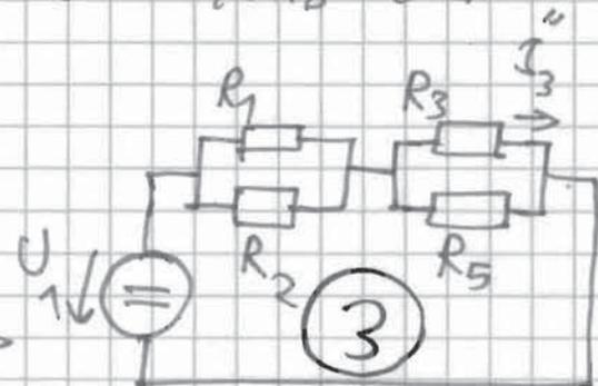
$$U_{R_3} = \frac{(R_5 || R_3)}{(R_1 || R_2) + (R_5 || R_3)} U_1 = \frac{(2R || R)}{(R || R) + (2R || R)} U_1 =$$
