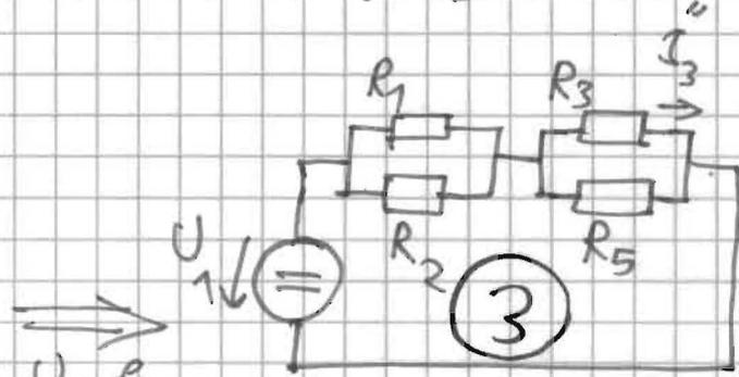
$$U_{R_3} = \frac{(R_5 \parallel R_3)}{(R_1 \parallel R_2) + (R_5 \parallel R_3)} U_1 = \frac{(2R \parallel R)}{(R \parallel R) + (2R \parallel R)} U_1 =$$
