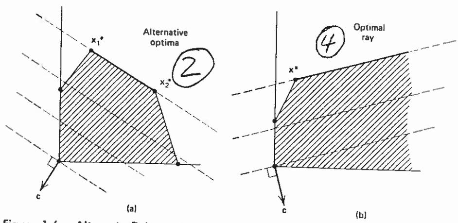
Figure 1.6. Alternate finite optima: (a) Bounded region. (b) Unbounded region.
