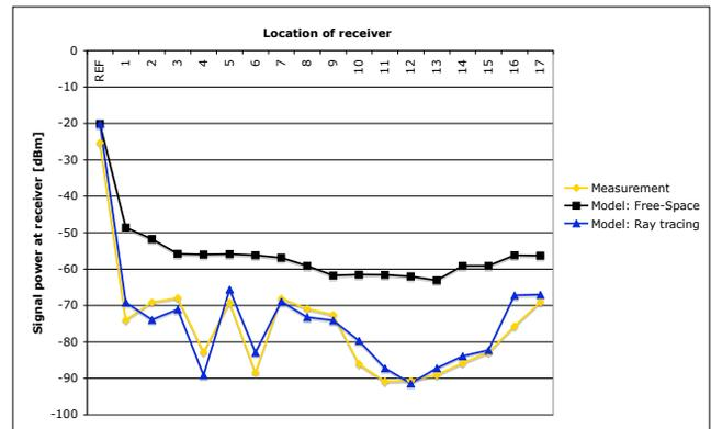
Figure 2: Experimental validation: State-of-the-art methods of VANET simulators overestimate the signal level in urban areas as they completely ignore buildings. Considering blockers and thus diffraction increases precision dramatically, as with only a crude approximation of the buildings the prediction by our ray tracing algorithm almost coincides with the measurement.
