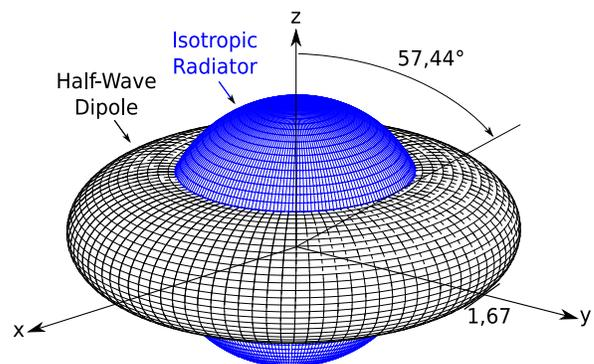
Figure 1: Direction-dependent gain of a half-wave dipole antenna (Equation 1) as compared to the ideal isotropic radiator: Between an angle of  $0^\circ$  and  $57.44^\circ$  the half-wave dipole's radiation is weaker than the one of an ideal isotropic radiator and higher between  $57.44^\circ$  and  $122.56^\circ$ . At  $90^\circ$  the half-wave dipole reaches its maximum gain and radiates 1.67 times as much power as an equally supplied isotropic radiator would do.
