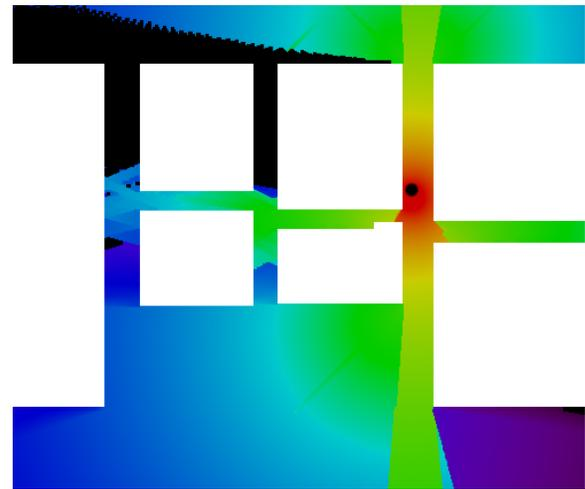
Figure 4: For the simulation buildings were modeled as cuboids. The false colors visualize the simulated path-loss (from red = small to blue = large).
