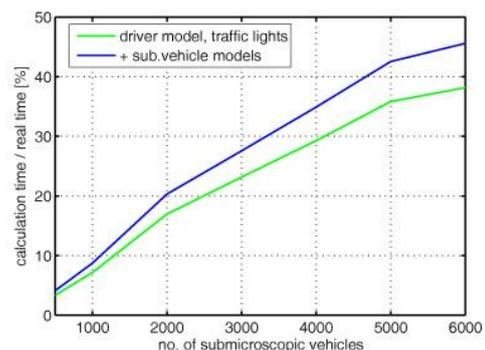
Fig. 5: Calculation time to real time vs. the vehicle number
