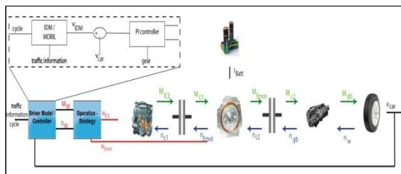
Fig. 2 Dynamic vehicle model, parallel hybrid
