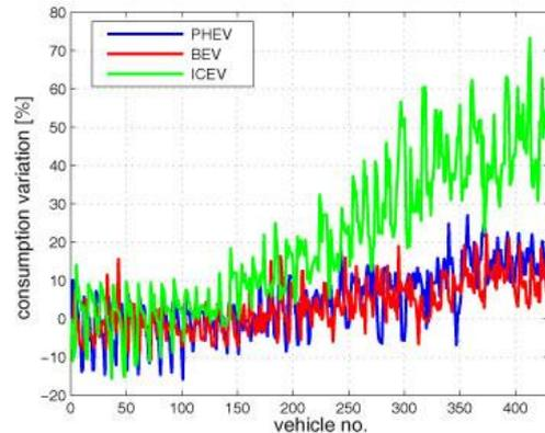
Fig. 3: Energy consumption in fleet traffic of PHEV, BEV and ICEV normalized to vehicle no. 1
