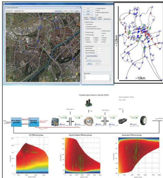
Fig. 4: ULTraSim graphical user interface and submicroscopic vehicle user interface for a PHEV with the motor / generator efficiency maps
