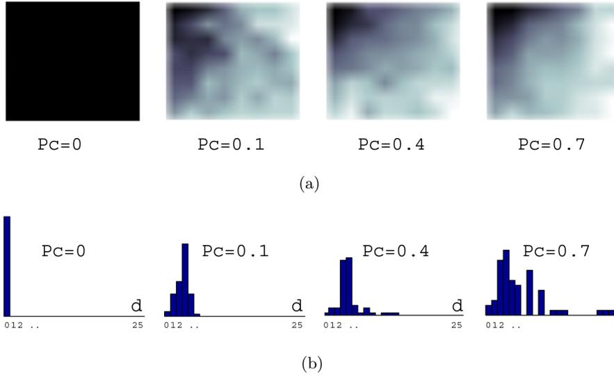
**Fig. 2.** Examples of simulation results with different link quality change probability  $P_c$ . (a) Delivery ratio at the end of different simulation runs. (b) Distribution of duplicates.
