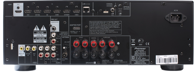
Figure 1: The figure shows the back panel of the amplifier used in our domain model and user study.
