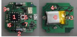
Figure 2. The Touchbugs PCB (upper and lower surface): (1) micro-controller; (2) left vibration motor; (3) rear LED; (4) right phototransistor; (5) button; (6) accelerometer; (7) gyroscope; (8) battery and (9) right colored LED.
