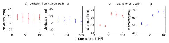
Figure 4. Results from two different experiments. The two leftmost graphs show the absolute deviation from a straight path for 5 different motor settings and 2 different lengths of bristles (red short, blue long). The two rightmost graphs show the diameter for circular motion (just one motor active).
