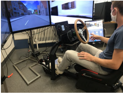
Figure 3: Driving simulator as used in the study. Situation 1 is currently displayed.
