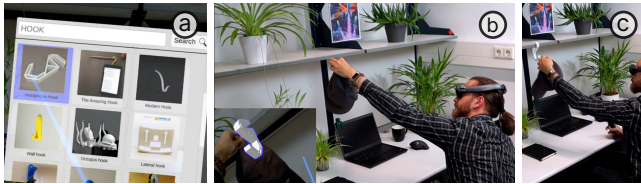
Figure 3: Brief workflow with Mix&Match: a) search for hook designs, b) in-situ preview of an appealing design, while coarsely verifying function and scaling it to fit (remixing), c) evaluation of the 3D-printed result.
