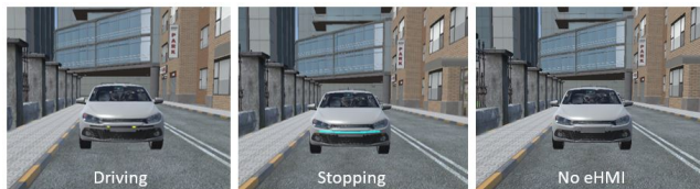
Figure 3: The three modes of eHMI that were operationalized by an LED band on the lower front of the vehicle: animated yellow dots represented driving (left), flashing turquoise band represented stopping (center), and no lights represented inactive eHMI (right).
