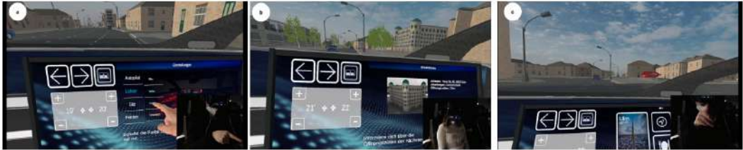
Fig. 1. Multimodal interface including touch (a), gaze (b), pointing (c), and voice inputs to refer to objects in and outside a vehicle.
