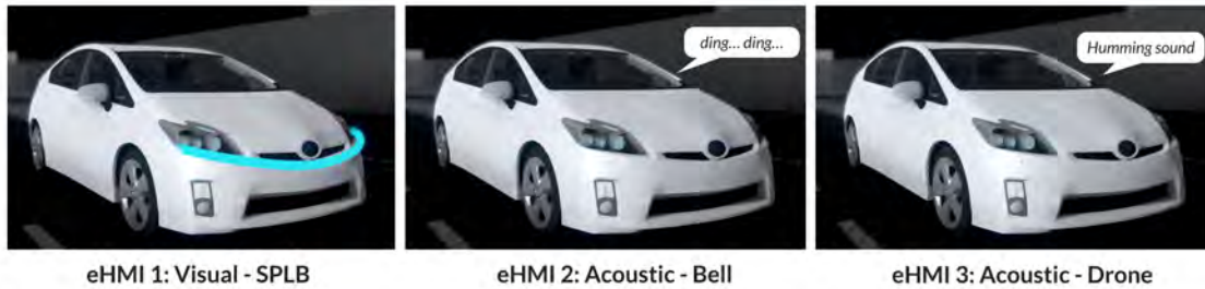
Fig. 1. We conducted a video-based study to test the effectiveness of 3 eHMIs: one visual (light-based: SPLB – Slow-Pulsing light Band), and two acoustic (sound-based: Bell eHMI that emits a dinging sound when the AV yields, and Drone eHMI that indicates a yielding intent by emitting a droning/ humming sound that changes pitch from high to low as the vehicle decelerates). Results showed that despite divergences in subjective opinions, the contrast between the eHMIs – individually or in combination with each other – had little effect on road-crossing decision objectively, indicating that once learned, eHMIs tend to work in general and design differences have relatively less impact. This leaves room for taking subjective user feedback into account in designing a pleasant user experience for eHMIs.
