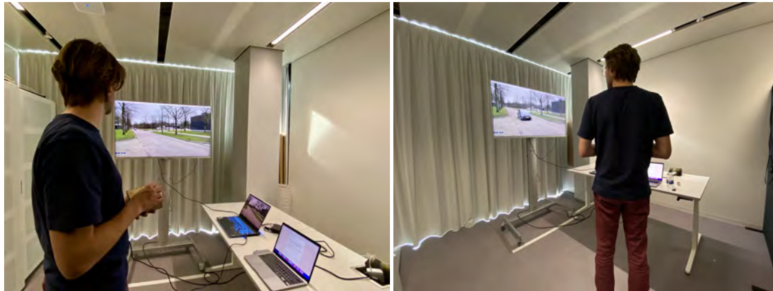
Fig. 2. The setup of the experiment: the participant stood sideways in front of a 55" screen where the video stimuli were presented.
