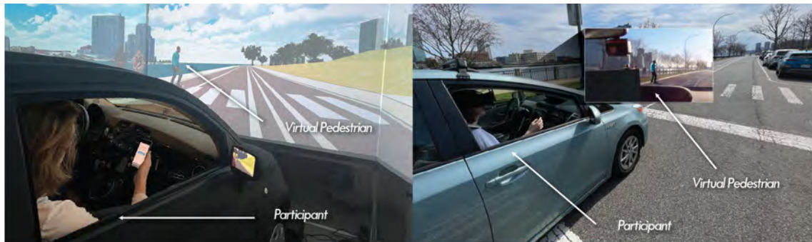
Fig. 1. Portobello enables platform portability , so that the same study can be run on in-lab (left) and on-road (right) driving simulation platforms.
