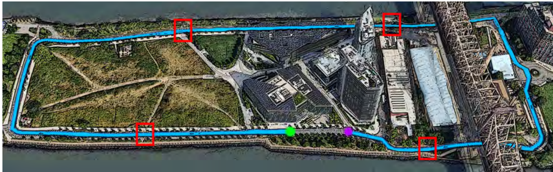
Fig. 4. Our study area for on-road simulator on Roosevelt Island. The pre-determined test route is highlighted in blue. The crosswalks with staged interactions are highlighted in the red bounding boxes. The start and end locations are denoted by the green and purple dots, respectively.
