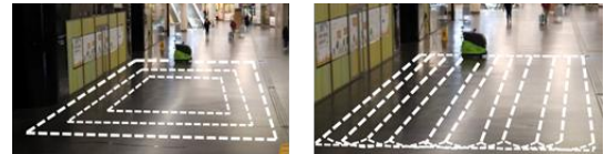
Figure 2. Observation of space and robot movement patterns. The white lines indicate the robots' movement patterns. The circular movement pattern (left); the off-set rectangular movement pattern (right).
