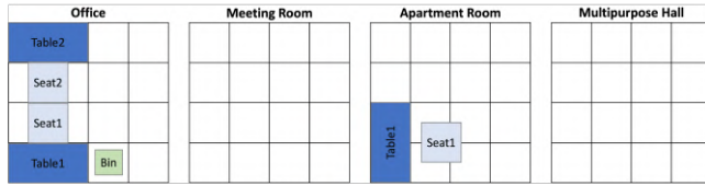
Figure 10: Schematic of the 2x2 m AirClick prototype used in the user study. Each panel shows a 4x4 ground-plate grid with the default arrangement of traditional furniture for the four scenarios: office, meeting room, apartment room, and multipurpose hall. The meeting-room and hall scenarios began with an empty grid. The drawn furniture blocks are scaled to roughly match their real-world dimensions.
