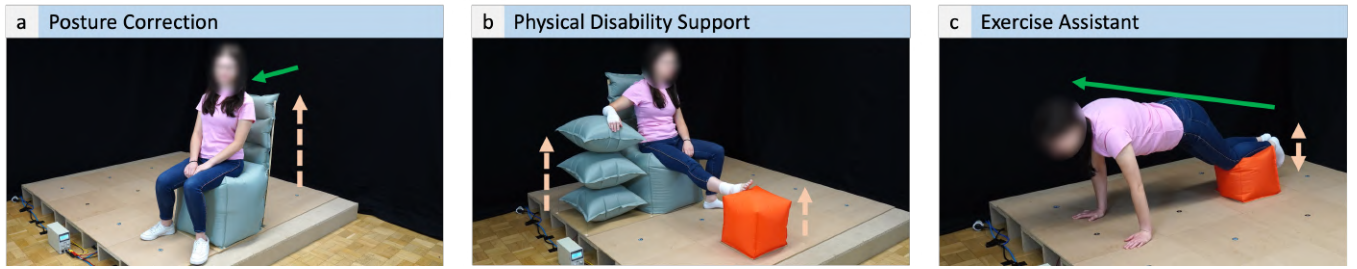
Figure 11: Health-promoting furniture application examples. (a) Automatic posture correction using a 1x1 chair with a separately activatable backrest. (b) On-demand support for arm and leg injuries using a reactive 1x1 cube and air-stack as arm and footrest. The cube inflates upon touching, and the air-stack inflates by holding the arm above the module. (c) Exercise assistant supporting a plank exercise by proactively inflating/deflating the module to adjust the difficulty.
