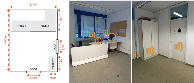
Figure 4: Left: Dimension of the real room and the object placed in it. Middle & right: Photos of the study room and the interaction space from the right back corner and the right front corner of the room. a) The cabinet that is recreated in the virtual scenario, b) The scented candle that creates the olfactory stimuli, c) The fan that creates the haptic stimuli, d) The doors that are placed in the same position in the virtual scenario.
