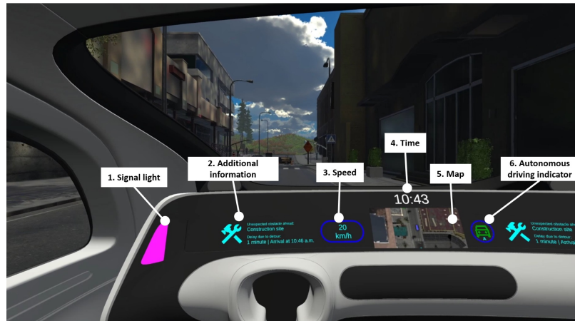
Figure 5: Dashboard of the AV. 1. Colored signal lights indicating normal driving-related actions of the vehicle via cyan and magenta for unexpected events, 2. information displayed on the dashboard, with large icons and text, 3. current speed, 4. time, 5. map showing surroundings, 6. autonomous driving indicator.
