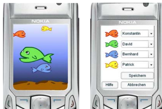
Figure 2. A screen saver where coloured fish are mapped to contacts and the corresponding configuration dialog. Parameters like speed, size and direction of the fish can be used to show communication patterns.
