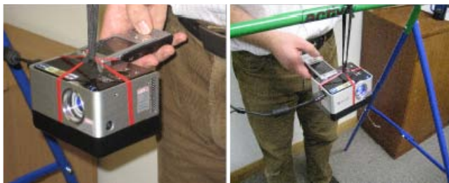
Figure 1. Prototype setup, N95 physically attached to a projector to simulate real use.
