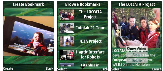
Figure 4. The Contextual Bookmark prototype on a Nokia N95. Left shows the view of the camera, centre a list of created bookmarks, and right the details of a bookmark.
