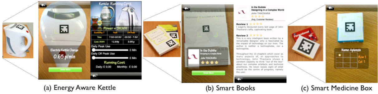
Figure 2: Prototype Smart Objects and Screenshots of Applications' Browsing Overlay Views and Detail Views
