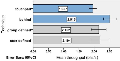
**Figure 7. Grand throughput of interaction techniques (since *group* and *user defined* yielded a comparably high error rate close to or above 10% their calculated throughput values may be less meaningful).**
