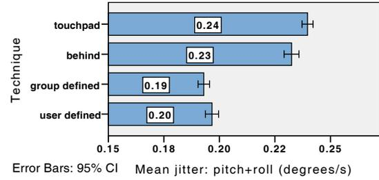
**Figure 8. Mean phone jitter (pitch+roll) measured as the sum of differences over time.**
