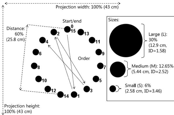
**Figure 3. ISO 9241-9 task. Visualization of size and height of projection in relationship to the three target sizes.**
