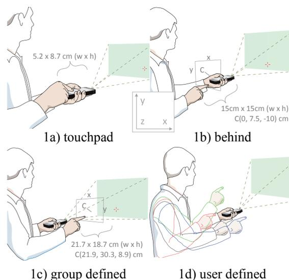
**Figure 1. Compared pointing techniques. ‘C’ denotes the central point of the interaction area in relation to the projector phone position (0, 0, 0).**
