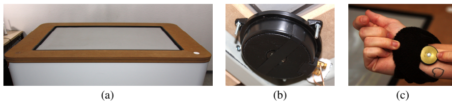
Fig. 2. The apparatus systems: (a) An interactive surface using rear projection. (b) Four 'bass pumps' mounted inside the interactive surface in order to generate low-frequency vibrations. (c) C2 vibration actuator to provide distal feedback.
