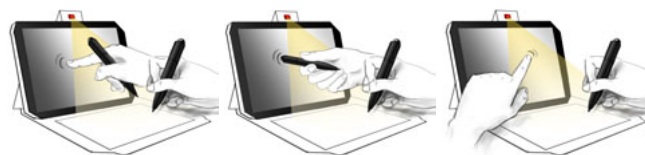
Figure 2. Interacting with the Penbook: (left) touch on the upright screen as well as pen-based input on the paper-based projection screen; (middle) pen-based input by using the rear side of the pen; (right) bi-manual interaction enables interaction with pen and touch simultaneously.
